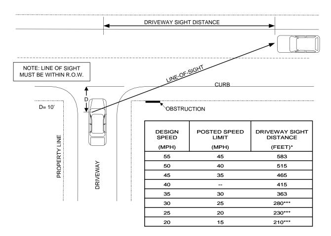
\* Driveway sight distance measured from a point on the driveway at 10 feet back from the edge of the road and measured from a height of eye at 3.5 feet on the driveway to a height of object at 4.25 feet on the road.
